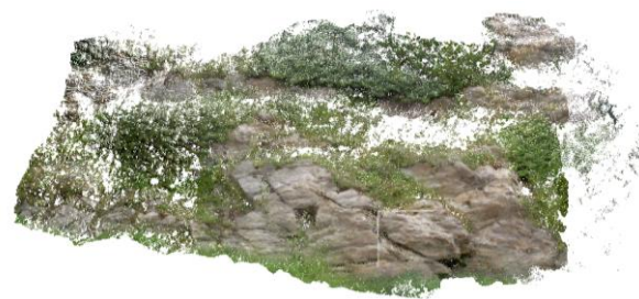
Figure 21. MicMac Konica dense point cloud
