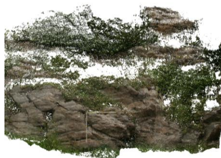
Figure 3. Dense point cloud for Canon5D, computed with MicMac. Vegetated areas show distinct holes.
