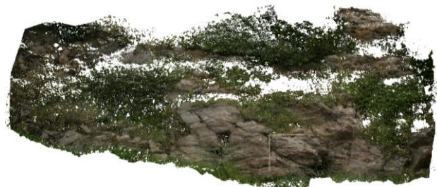
Figure 20. MicMac Canon5D dense point cloud
