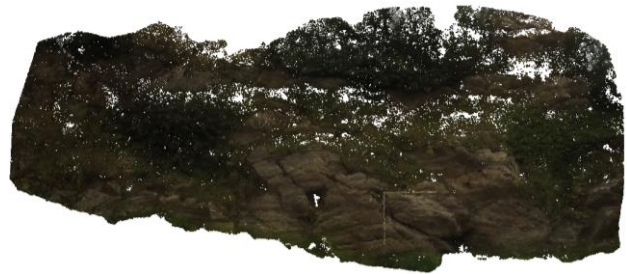
Figure 11. Pix4D GoPro dense point cloud
