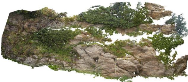
Figure 8. Agisoft PhotoScan Smartphone dense point cloud
