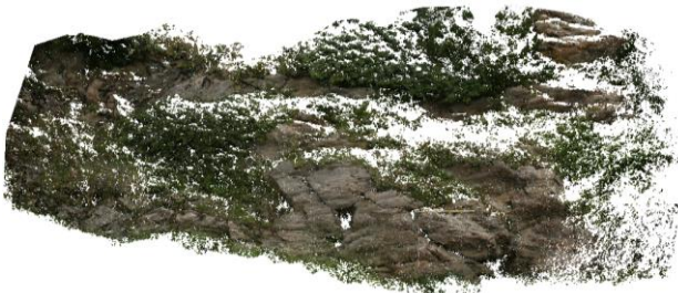
Figure 15. SURE Canon5D dense point cloud
