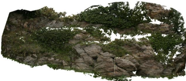
Figure 5. Agisoft PhotoScan Canon5D dense point cloud
