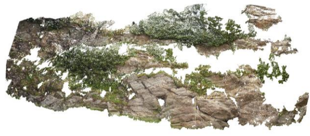
Figure 13. Pix4D Smartphone dense point cloud
