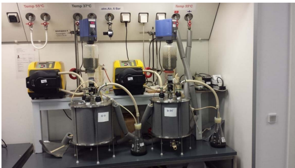
Figure 1. CSTR experimental set up used for the anaerobic co-digestion of urban organic waste (Fitamo et al. I , Supplementary Information).
