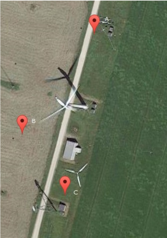
Figure 10 - The position of three wireless mics during test measurements around the Nordtank test turbine during the summer of 2016. Three test positions around the test turbine were chosen: A - equipped with BSWA Mic no. 1 and Wi-Fi mic A; B equipped with BSWA Mic no. 5 and Wi-Fi Mic B, and C equipped with BSWA Mic no. 4
