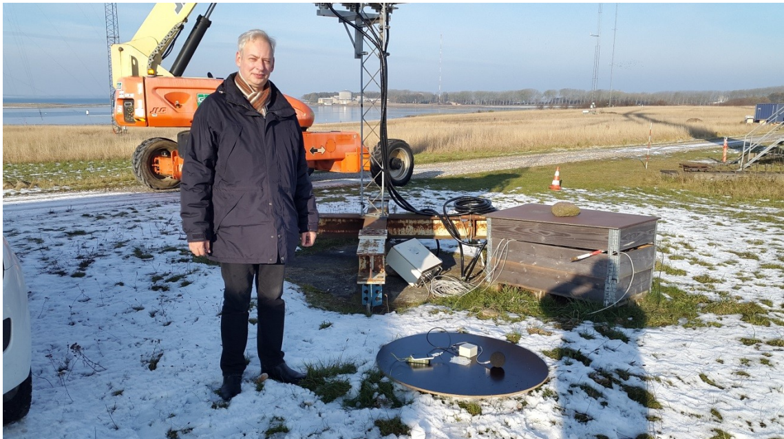
Figure 9 - Steen Sørensen DTU/TEM in the test field next to one of the 42 wireless mics during testing at Campus Risø in November 2016. On the plate is seen: One mic with B&K wind sock connected to a Nokia mobile telephone and a battery package. This autonomous WIFI network connected mic system. With the battery package shown each of the autonomous GSM network controlled mic systems is able to record and transmit time series of noise measurements continuously for a 12 hour period.
