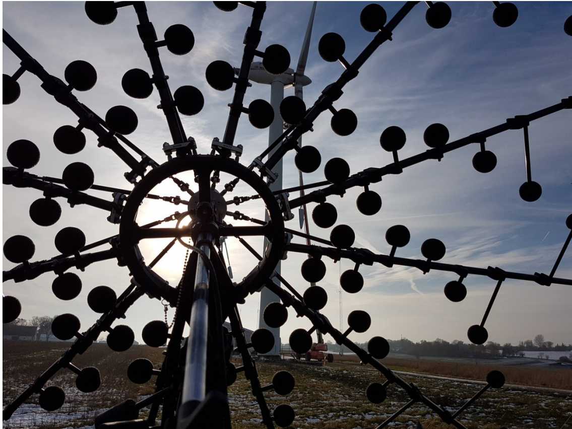
Figure 12 - The FlexStar 120 mic acoustic antenna of 4 m diameter developed and deployed at Risø campus by GFai Berlin simultaneously with test activities with wireless mics at DTU Campus Risø, Nov. 2016.
