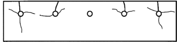
Figure 12: Typical crack patterns in test specimens subjected to accelerated corrosion, from [24].
