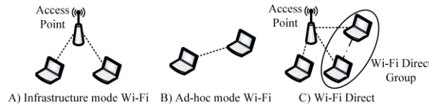
Fig. 2. Different modes of Wi-Fi deployment
