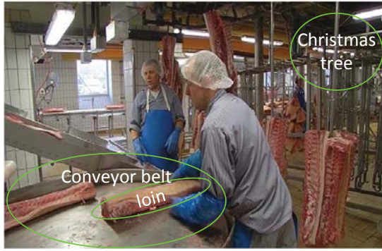
Fig. 2. A pick and place task in slaughterhouse: the target object loin has to be grabbed from the conveyor belt and transferred to the hook on a metal Christmas tree.
