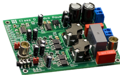
Fig. 11: Implemented 12 V test amplifier.
