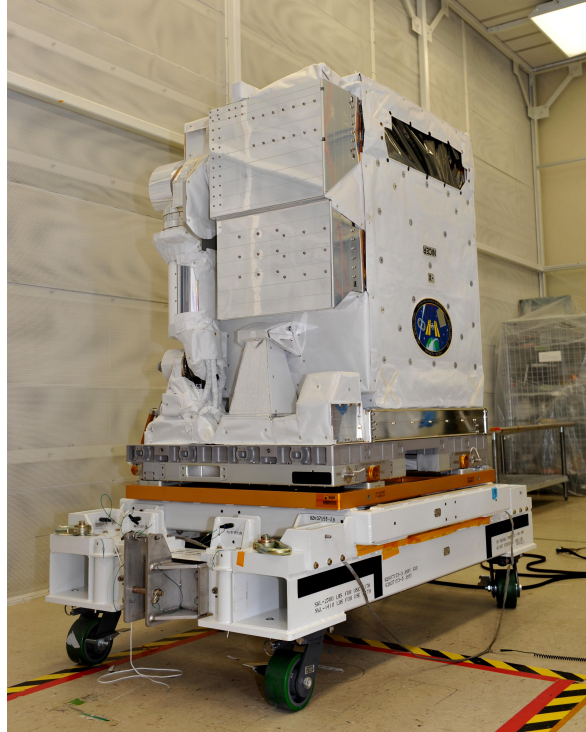
Figure 2. The NICER flight payload in a nearly fully integrated configuration, blanketed and stowed against the flight A-FRAM plate.
