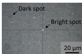
Figure 2.8: Optical micrograph used for determining where to do a Raman measurement. A typical "bright spot" and "dark spot" are indicated.
