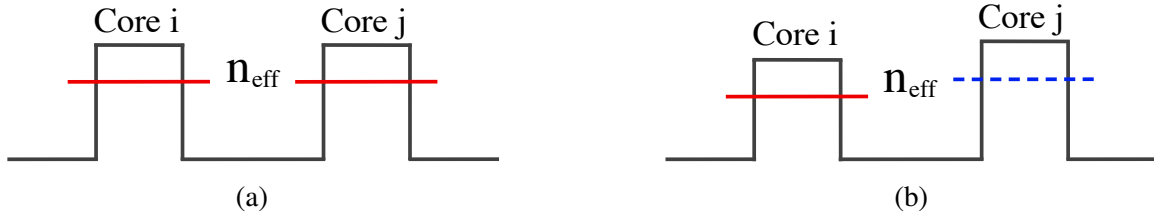
Figure 2.7: Refractive index profiles and corresponding effective indices in (a) a homogeneous core arrangement and (b) a heterogeneous core arrangement.
