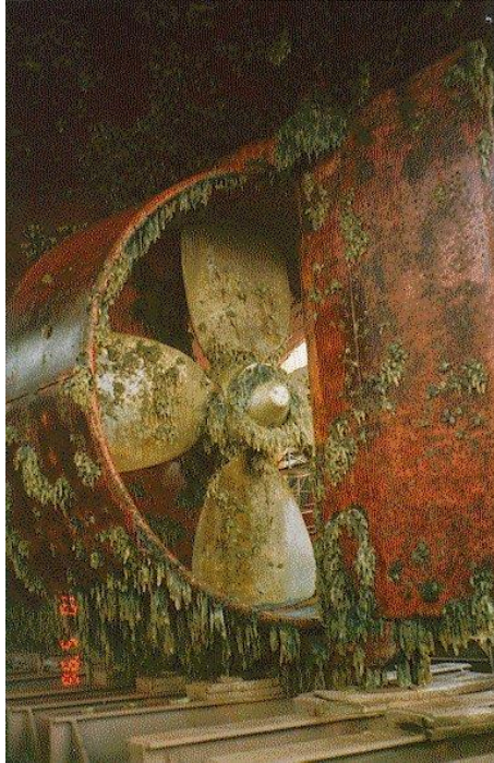
Figure 1.1. Biofouling settlement on the propeller of a vessel. Courtesy of Hempel A/S.
