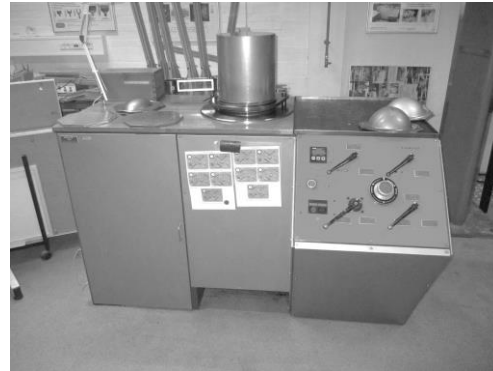
Figure 3. In-house build bulge tester.
