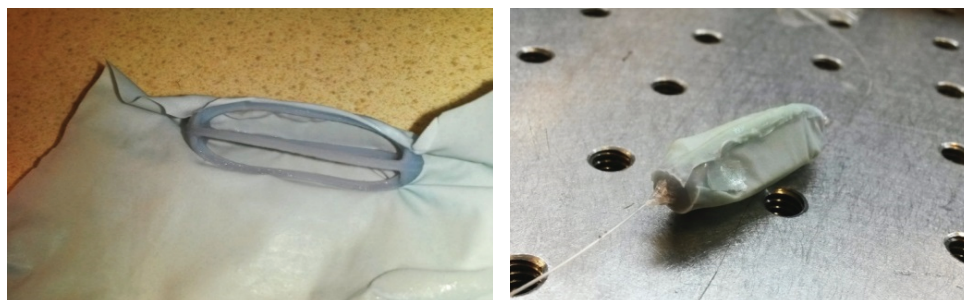
Figure 6-8. Wrapping of the transducer pod in latex cloth (left) and the complete pressure sensor (right)
