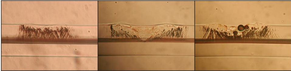
Figure 3-4. Fibre after 30 min of 325 nm UV laser FBG inscription on 3 different fibre sections
