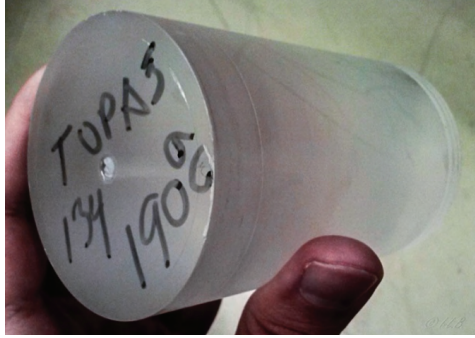
Figure 1-2. Preform for polymer step-index fibre (presented with permission from Andrea Fasano). The cladding was made of Zeonex 480R. The core is 4 mm in diameter, material was TOPAS 134C, it was injection moulded inside the cladding material.
