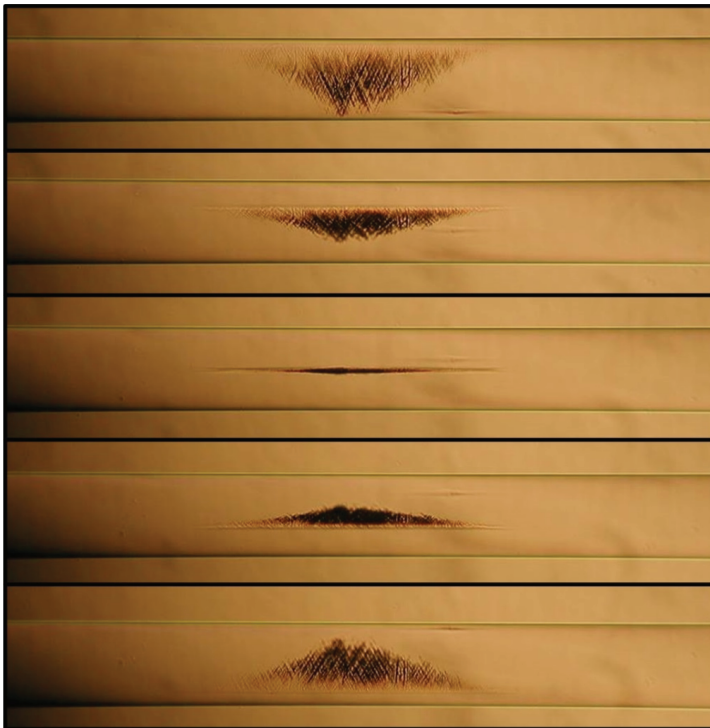
Figure 3-2. Images of a burned bulk dummy fibre, taken at different rotational position of the fibre. This fibre was around 150\ \mu\text{m} in diameter thick, it was used for alignment purposes and irradiation duration determination. The grating used for making an FBG in our setup forms two orders +m and -m , these orders are clearly visible in this burned fibre
