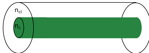
Figure 2.1: Sketch of a simple step index fiber, where the refractive index of the core, n_c , is larger than the refractive index of the cladding, n_{cl} .
