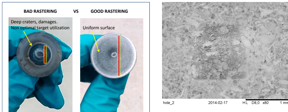
Figure 5.4: Left: Bad rastering VS good rastering. In red is depicted the corresponding rastering path. Note that the laser beam passes right close to the center, but not exactly by the center to avoid target damaging related to excessive \frac{\#pulse}{u.area \times u.time} as discussed in the text. Right: SEM image of target damaging as consequence of laser ablation. The morphology keeps worsening as the number of pulses increases.
