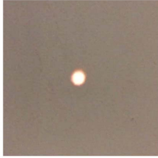
Figure 5.10: First video frame of the spatially dithered focused beam ( \omega_0 = 1.56 \text{ mm} ) at probe range R = 60 \text{ m} . The video (see Visualization 1 ) is slowed down four times the original speed to show the beam’s spiral trajectory.
