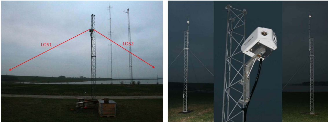
Figure 6.2: Images of the experiment, where WindEye1 is compared with 2 sonic anemometers. The instruments are placed such that the sonic measurement volume is within 0.3 m of the lidar beam, and the distance between the sonic anemometers and lidar matches exactly to the respective weighting function peak position. Adapted from [67]
