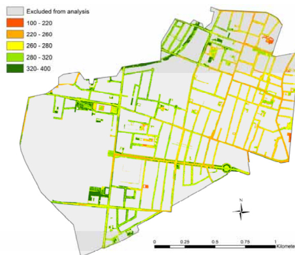
Figure: Site suitability scores for permeable pavement placement in Frederiksberg, Denmark
