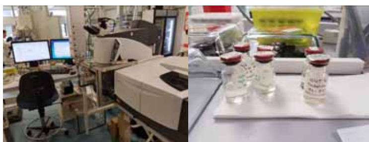
Figure: The FT-IR imaging machine (left). Microplastic particles concentrated in ethanol
