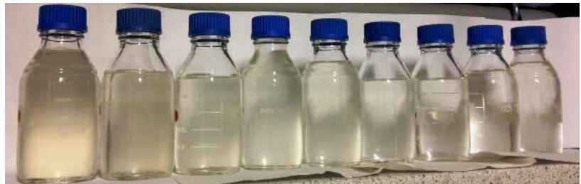
Figure: Clarity of greywater from inlet to outlet of each box
