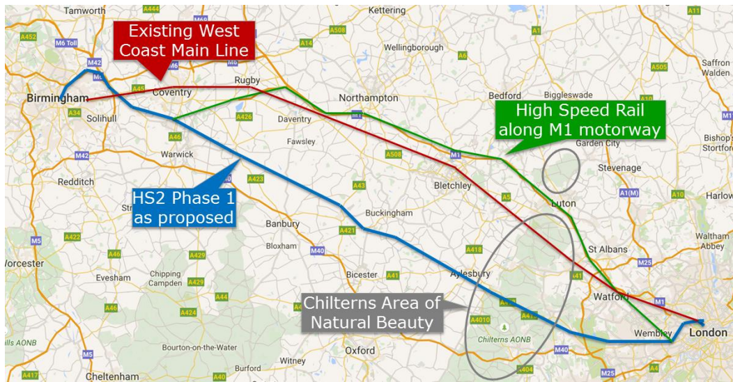
Figure 2: Alternatives along existing transport corridors considered for HS2 Phase I: Slower route along the M1 motorway (green); Upgrade of the existing West Coast Main Line (red).
