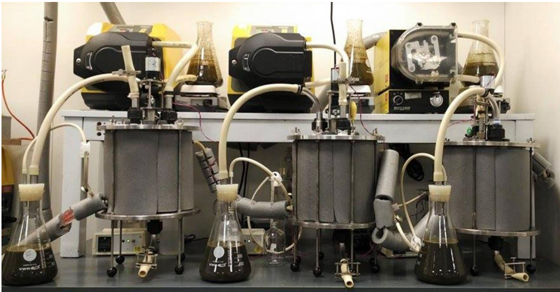
Figure 6. System set up for the bioaugmentation with hydrolytic microbes during the co-digestion of wheat straw with cattle manure.
