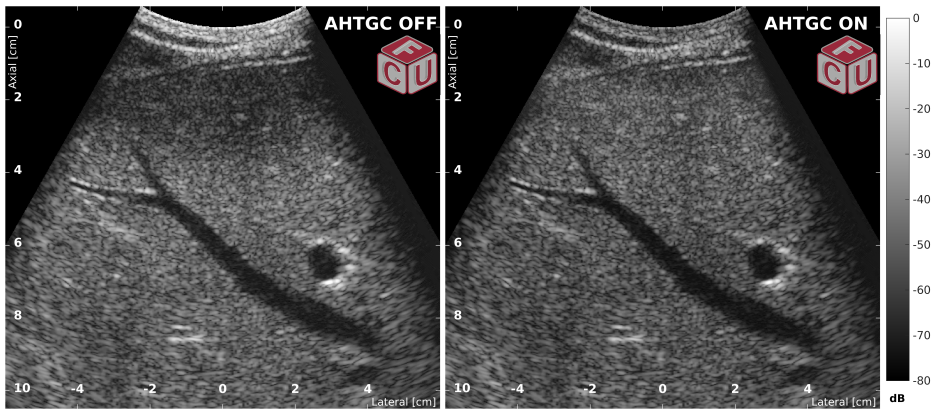
(b) Result of AHTGC applied to an axial view of a human liver. The Image on the left is adjusted by the factory preset TGC with no default gains, and The image on the right is processed with AHTGC.
