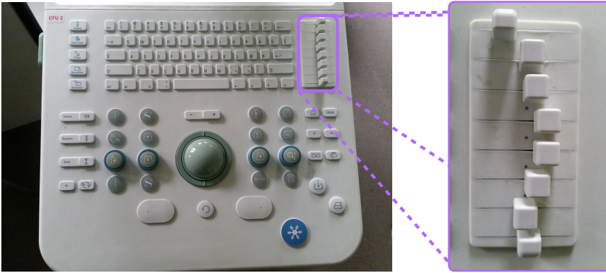
Figure 1.1: The keyboard of a commercial ultrasound scanner. The zoom-in shows the TGC gain sliders.
