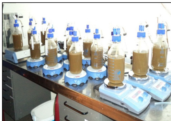
Fig. 2. Anoxic/anaerobic 1 L batch reactors used in the experiment.
