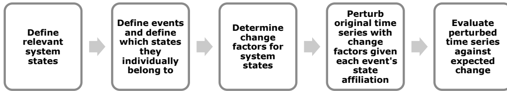
Figure 1. Flow diagram showing the general process involved in the presented methodology.
