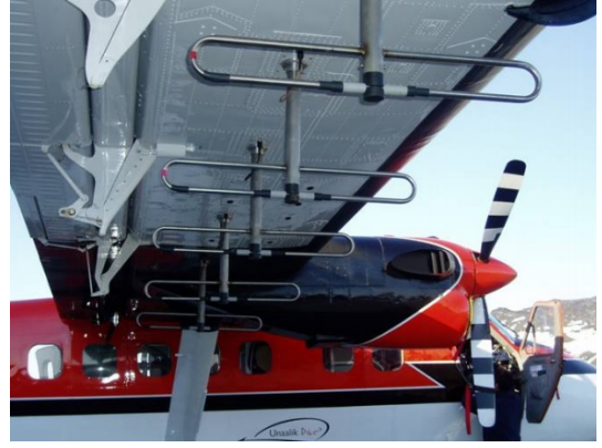
Fig. 1. A photograph showing the 5-element sub-array of folded dipole elements mounted under the right wing of the Twin-Otter aircraft.
