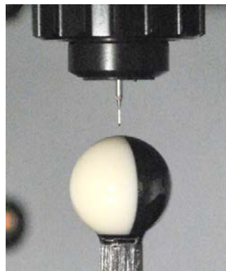
Figure 2. Example of a multi-material sphere, \text{Al}_2\text{O}_3 (white)/ \text{Si}_3\text{N}_4 (black) multi-material sphere, assembled in a high precision tactile CMS
