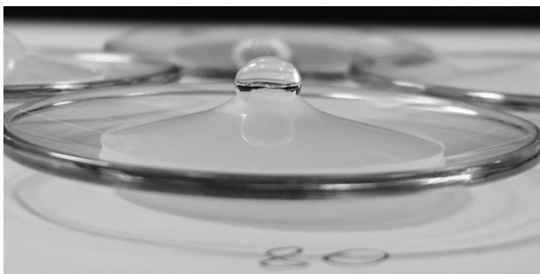
Figure A-3.1.3. Water droplet on top of a crosslinked 25 mm in diameter G80_S184 disc sample after approximately 1 hour.
