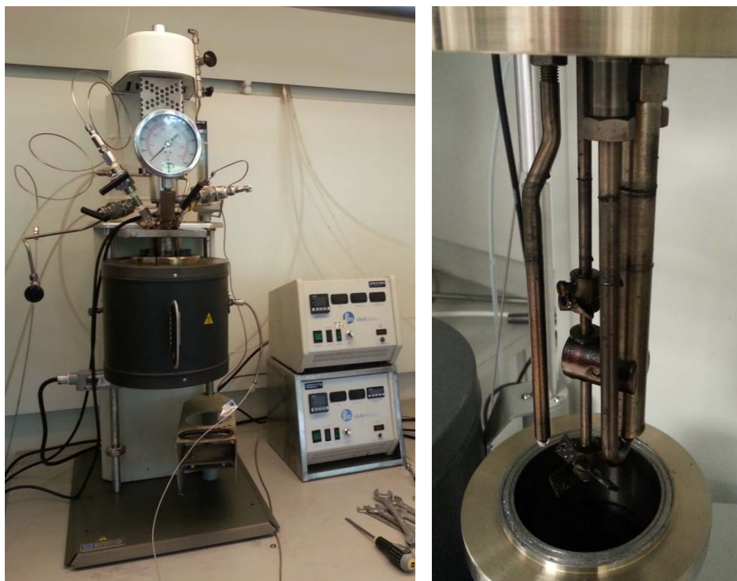
Figure 3.1 The experimental setup used for all of the experiments. Left: The assembled batch reactor with the heating jacket mounted. Right: The internals of the reaction vessel comprising of sampling tube, stirrer, cooling coil and thermowell seen from left to right.
