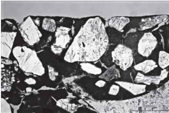
Figure 5. Enlargement of the section of the medieval mortar. The “R”s show cracks. Transmitted light. No filters. Dark colour is lime binder. Top of the picture is the outside surface with the dense calcium carbonate layer. (Photo: SEIR-materialeanalyse A/S)
