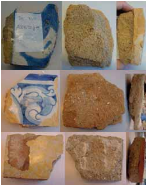
Figure 4: experimental tiles with mortar. Top: 17 th century tile from Alentejo (PT); middle: 18 th century tile from Palacio Centeno, Lisbon; bottom: 20 th century tile of unknown origin.
