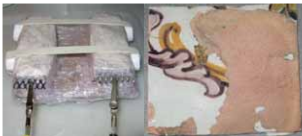
Figure 3: (a) Experimental setup for desalination of single tile; (b) 20 th century tile used in lab experiment.
