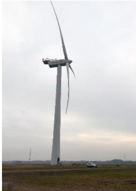
Figure 28. Running of the turbine while measuring the deformations.
