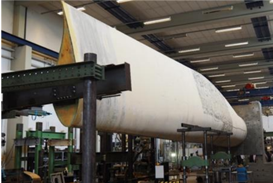
Figure 44: Full test setup for handling of the 15m inner root section of the SSP34m blade: a) 3D illustration and b) photography representation
