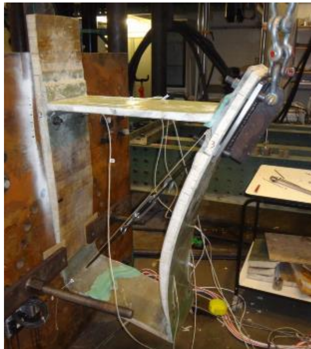
Figure 124: Sub-component test of the rear box of the 60m blade range with the X-Stiffener technology.
