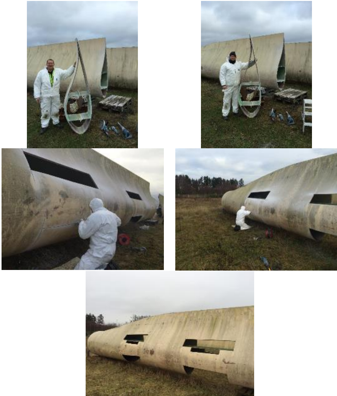
Figure 40. Cutting out of different blade specimens.
