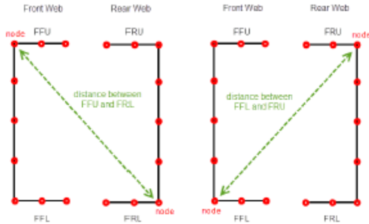
Figure 116: Webs' FE mesh, node location. FFU-FRL and FFL-FRU distances definition.
