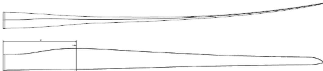
Figure 104: Main features of AB6X blade – AB6X edgewise and flapwise views.
