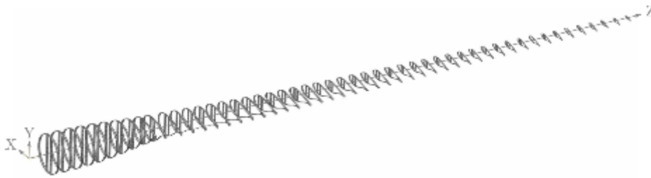
Figure 83 - Baseline cross sections and coordinate system of DTU 10 MW reference wind turbine rotor blade.
