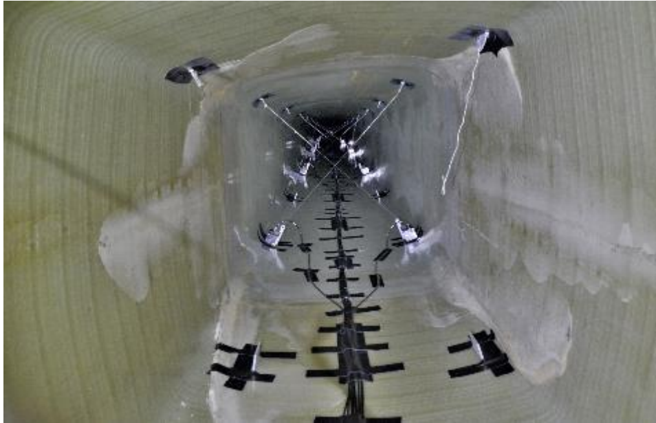
Figure 26. Inside of the blade mounted with measurement equipment.
