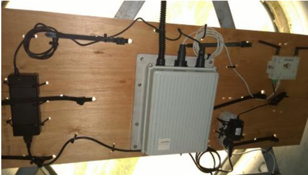
Figure 19: The WindMETER system mounted centrally in the hub with the power unit on the left, and data transmitter on the right.
