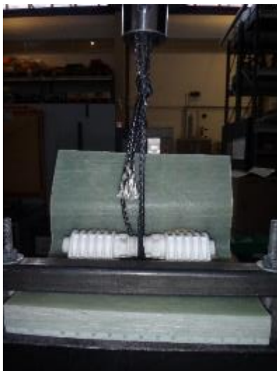
Figure 7: Mechanical test of the X-Stiffener at DTU Mechanical.
