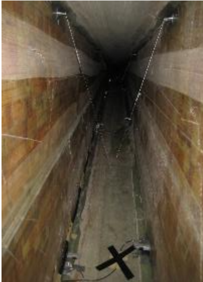
Figure 36. Inside of the blade mounted with measurement equipment.
