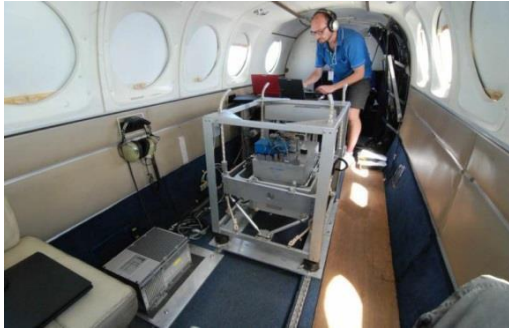
Figure 2. The Imar-IMU unit and LCR S-99 gravimeter.
