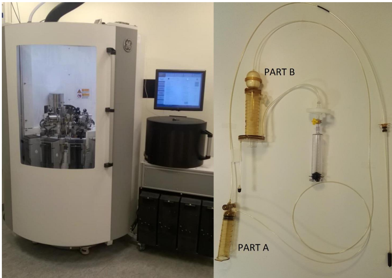
Figure 11: SPINlab and fluid path for clinical use, consisting of Part A and Part B.
