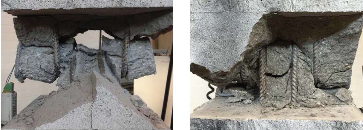
(a) With precast dowel
