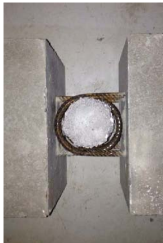
(b) Positioning of dowel
