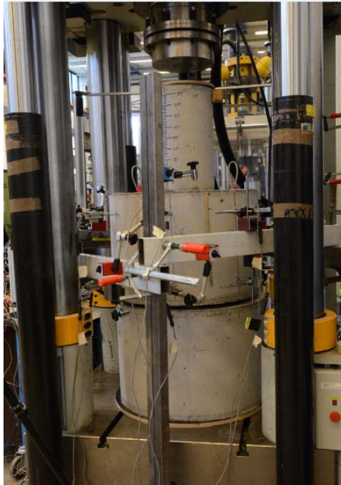
Figure 10: Test specimen on concrete base placed in 5 MN INSTRON machine.
