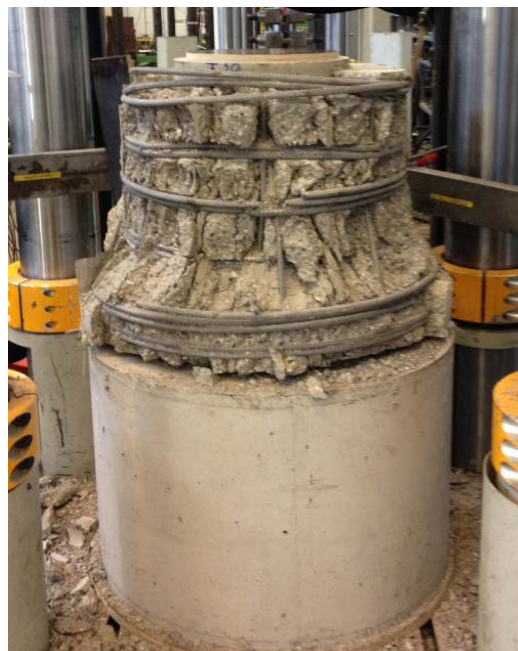
Figure 17: Crushing of piston before yielding of stirrups in sleeve of specimen 5-H-D (top) and damages of sleeve in specimen 6-H-W after ca. 480 mm piston displacement (bottom)
