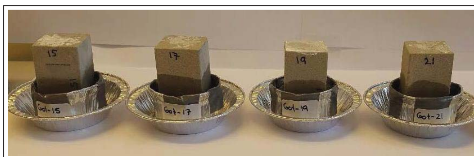
Fig. 3: Suction test after ED.
