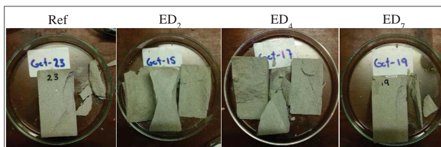
Fig. 7: The stones after compressive strength measurements.
