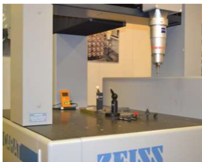
Figure 6. Zeiss UPMC 850 tactile CMM used as calibration equipment within the comparison
