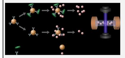
Using 250 nm "ghost" magnetic nanoparticles, which widen the linear detection range of 100 nm magnetic nanoparticles, the performance of the optomagnetic sensor system for the quantitative analysis of target DNA sequences (through binding of DNA-tagged magnetic nanoparticles to rolling circle amplification products) and bacteria (direct immunoassay protocol) is improved by a factor of 15 compared with the classical approach excluding ghost nanoparticles.
