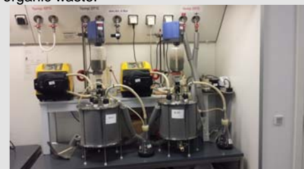
Experimental set-up of co-digestion process in continuous stirred tank reactor
