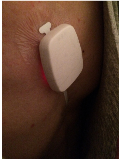
Figure 4.14: PPG-patch at the sternum (the red light illuminating the skin is also seen).
