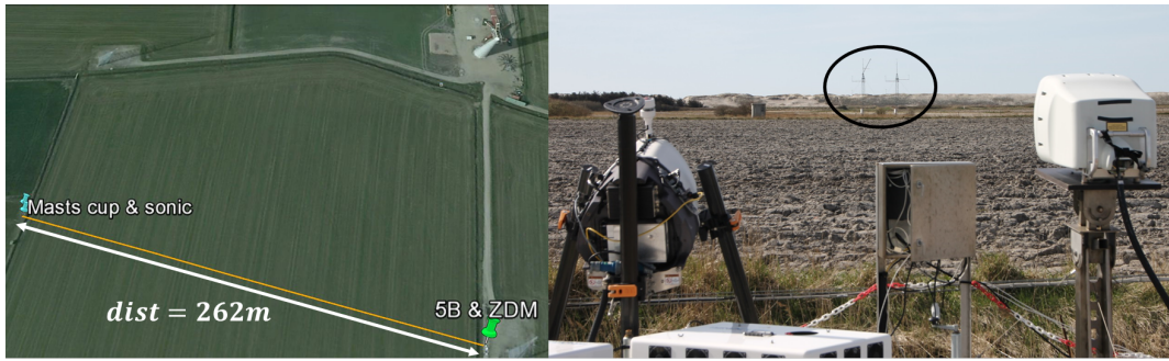
Figure 5. Calibration measurement setup at DTU Wind Energy's test site, Høvsøre, Denmark. Left: Google Earth image; Right: the ZDM and 5B lidars.
