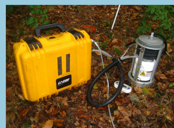
Figure 1 (left): One of eight automated soil respiration chambers (8100-104 Long-Term Chamber, LI-COR Biosciences).
