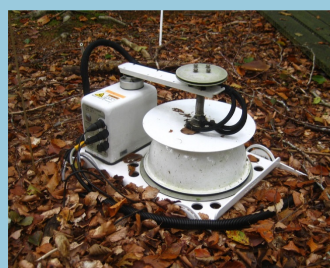
Figure 1 (left): One of eight automated soil respiration chambers (8100-104 Long-Term Chamber, LI-COR Biosciences).
