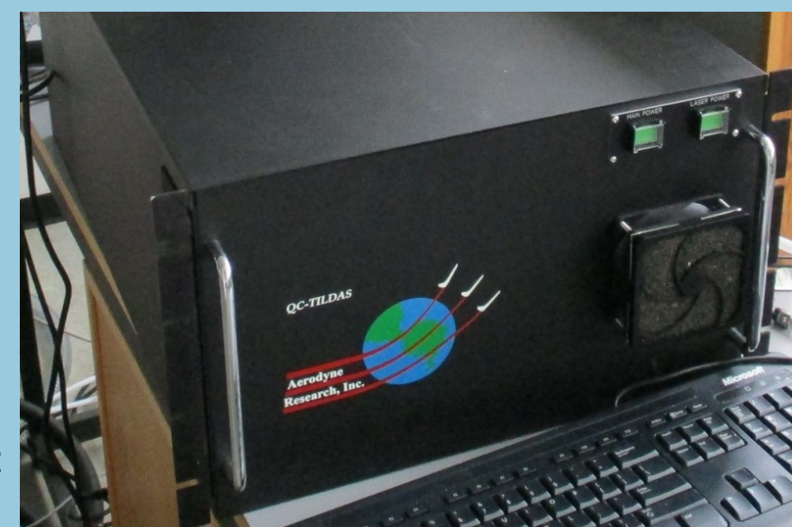
Figure 2 (right): The Aerodyne Single CW-Quantum Cascade Laser Trace Gas Analyzer for CO 2 Isotopes (Aerodyne Research Inc.).
