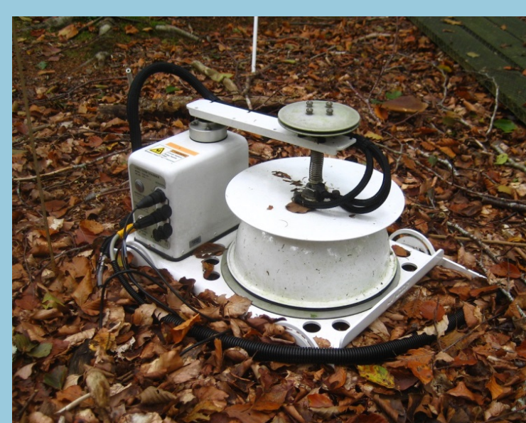
Figure 1 (left): One of eight automated soil respiration chambers (8100-104 Long-Term Chamber, LI-COR Biosciences).
