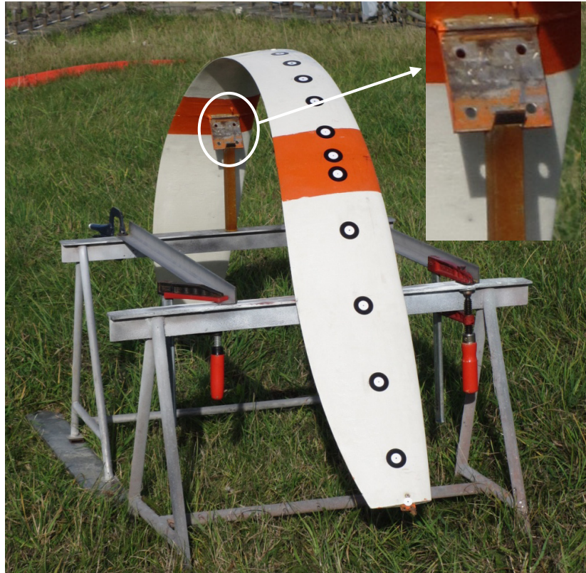
Figure 3.10: Blade and hinges configuration
