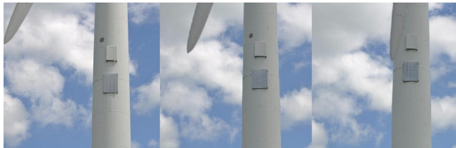
Figure 6.7: Position of the pattern while the blade is passing in front of it
