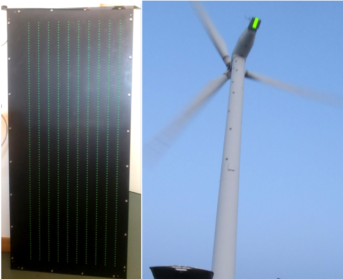
Figure 6.14: LED array designed for the BOS experiment
