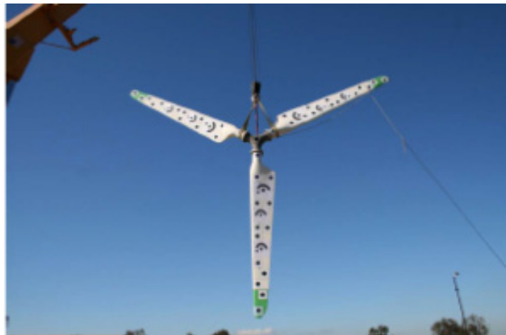
Figure 1.3: Point tracking markers on wind turbine rotor for investigating the effects of seismic activity. UCSD, California [thanks to Tim Schmidt Trillion, USA]
