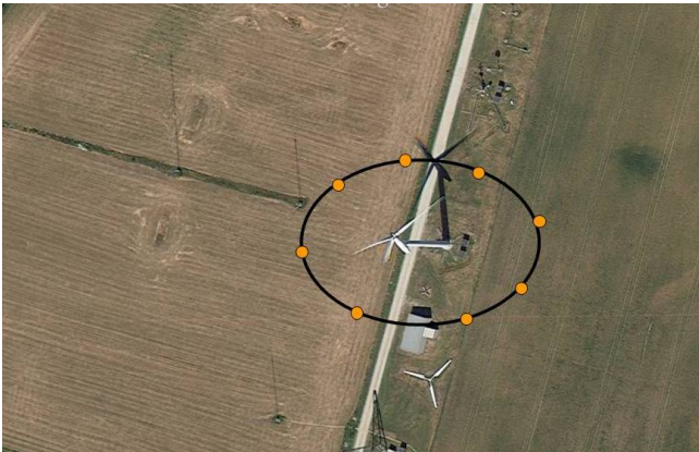
Figure 3. The 8 microphones on the ground positioned around the turbine on a circle at equidistant angle intervals.
