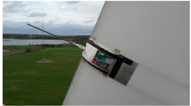
Figure 7. The autonomous inflow sensor unit mounted on the blade.
