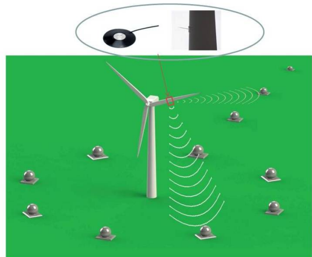
Figure 1. Sketch of the experimental set-up. Surface microphones on one of the blades and a five hole pitot tube for inflow measurements. On the ground eight microphones on plates at equidistant angle intervals around the turbine in a radius of one rotor diameter. Finally, a number of wireless microphones in the far field beyond one rotor diameter for noise propagation measurements (not used in the present campaign).
