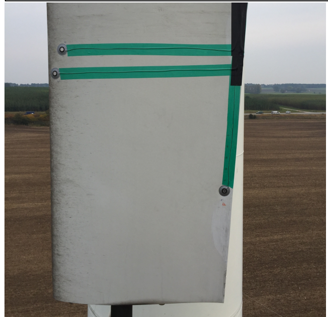
Figure 9. The microphone positions in campaign II. Two microphones were at the LE and one at the TE on each side of the blade. The photo shows the microphones on the pressure side.
