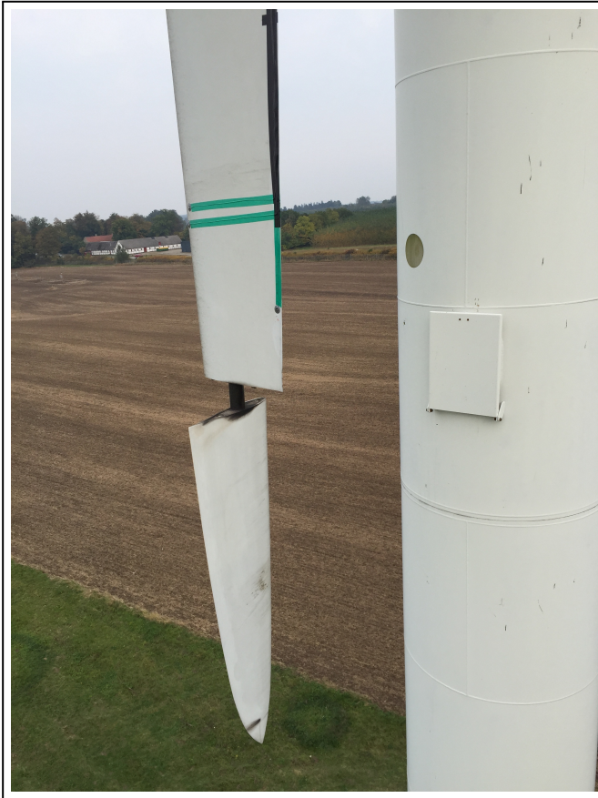
Figure 5. Photos showing one of the surface microphone set-up's as used in the measurement campaign II. Two microphones close to the LE.(5 and 10 chordwise position) and one microphone close to the TE (95 chordwise pos.) on both the pressure and suction sides of the blade.
