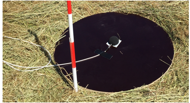
Figure 6. One of the eight microphones around the turbine on the plywood board and with a wind shield.
