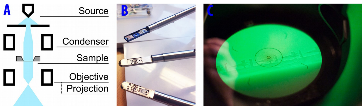
Figure 3.1: A: Simplified schematic of the optics in a TEM. A homogeneous irradiation strikes the sample. By focusing the objective lens on the sample an image can be projected onto a screen below. B: Three variations of modern chip based TEM-holders (designed, built and photographed by Murat Yesibolati). C: The projected image can be visualised by means of a phosphor-screen at the bottom of the TEM. Here a set of MEMS devices being characterised by Alexey Savenko.
