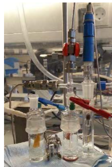
Figure 1: Liquid cell for measurement of CO 2 reduction products. Shown here with a Cu sheet electrode as electrocatalyst.
