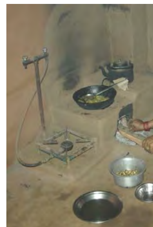
Figure 1: Cooking technology alternatives in rural setting: a biogas stove & an improved woodstove.
