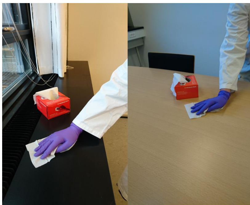
Fig. 9 Dust sampling using clean precision Kimwipes® Lite wipes from regularly cleaned surfaces
