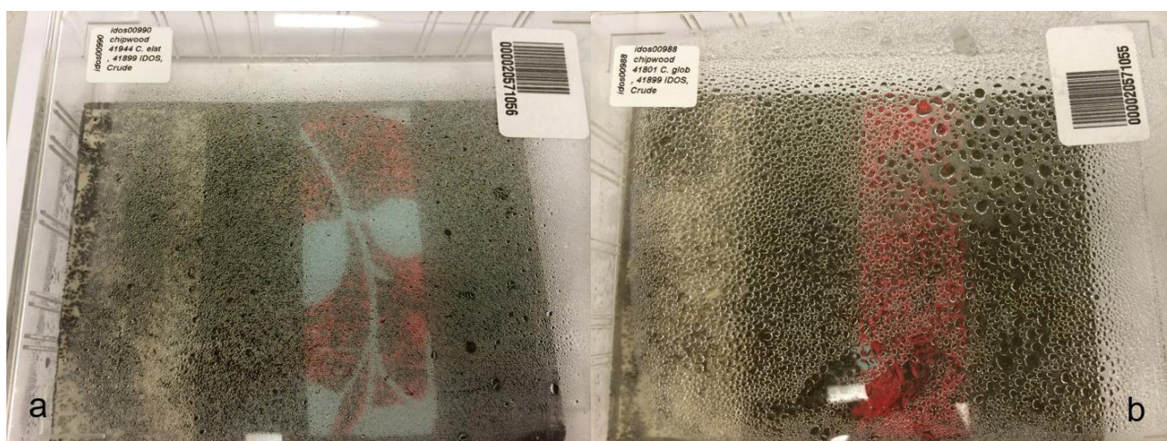
Fig. 19 Occurrence of condensate as the result of fungal degradation of chipboard: a – C. elatum (IBT 41944); b – C. globosum (IBT 41801)
