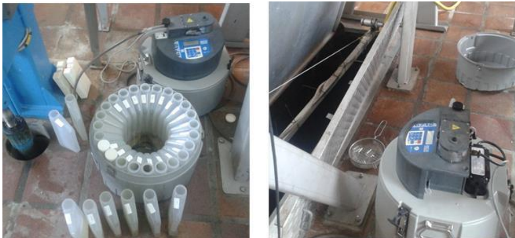
Figure 5.2 An automatic sampler in time-proportional mode during 2-week sampling campaign from raw influent after screening in Lynetten WWTP. The sampler included 24 bottle (left) allowing collection of hourly composite samples. At the end of each sampling day, hourly samples were mixed flow-proportionally to make 6-hourly samples. TSS was also measured during sampling using sensor (right).
