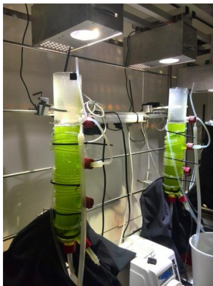
Figure 17: The 1.4-L PBRs used in continuous cultivation. The light was supplied only from the top of the reactor and the reactor walls were covered with black cloths to avoid light entering from the side.
