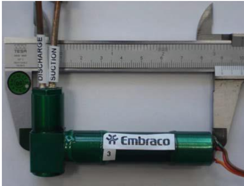
Figure 2.9 Compressor: 9 cm long, compression ratio = 2.4. (Mongia et al. (2006)) © [2006] IEEE.
