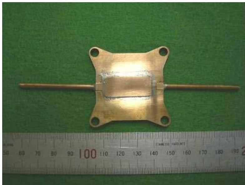
Figure 2.10 Microchannel evaporator: Cooling load 40W, edge = 5 cm. (Mongia et al. (2006)) © [2006] IEEE.
